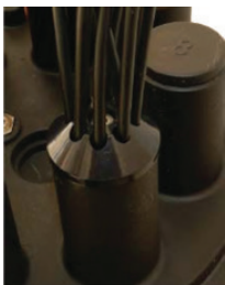
Drop cable sealing
